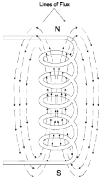
Figure 3 - The magnetic lines around a current carrying conductor leave from the N-pole and re-enter at the S-pole.
